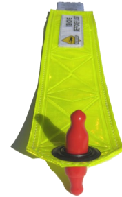
The PSDASP0908 is a diamond stall warning plug. The Plane Sights double-sided stall warning plug fits any Diamond DA40, DA50 and DA20, one way or the other.
